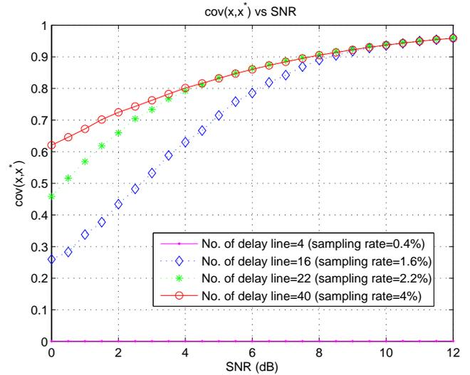
Fig. 6. Covariance between the original signal and reconstructed signal.
