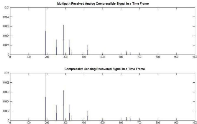
Fig. 5. Original signal vs. CS recovered signal.
