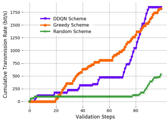
FIGURE 12. The number of validation iterations versus cumulative transmission rate from eNB to the vehicle relay.
