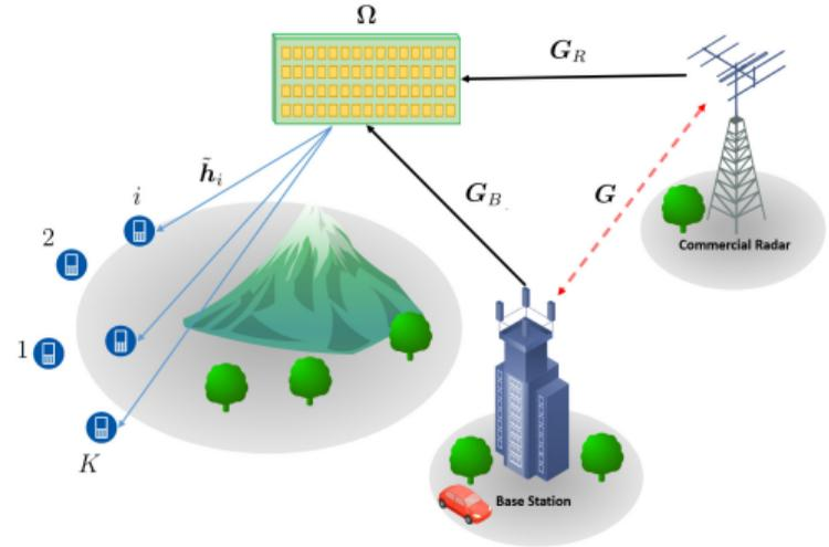
Figure: RIS-assisted MIMO RCC system
