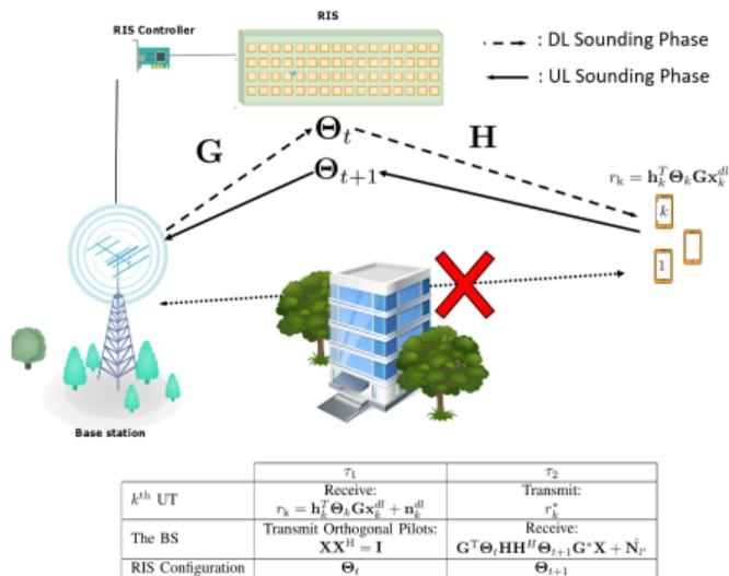
Figure: System Model for RIS-Assisted MU-MIMO Communication System.
