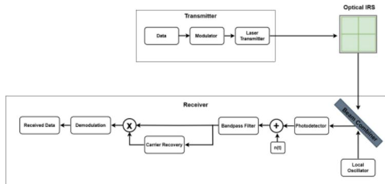
**Figure:** System model for IRS-assisted Coherent OWC system.
