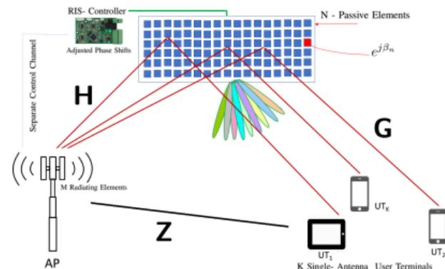
Figure: RIS- Assisted massive MIMO system
