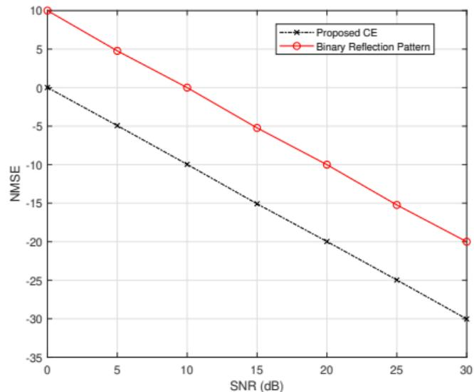
Figure: The performance of FR method on estimating the LOS channel vs different SNR values.
