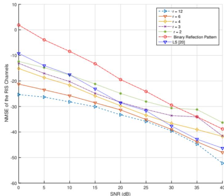
**Figure:** The Effect of Sub-RIS size on the NMSE performance vs SNR.
