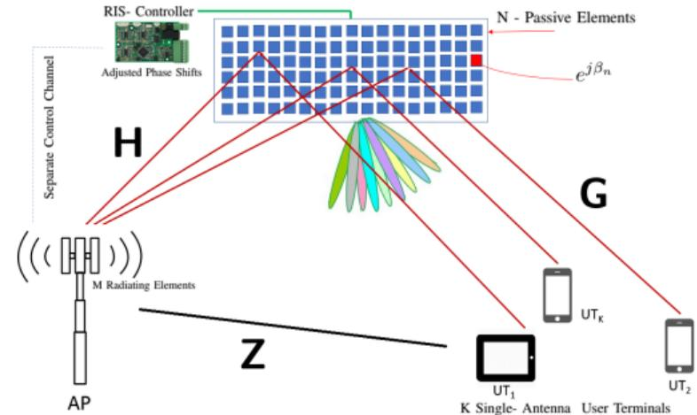
Figure: RIS- Assisted massive MIMO system
