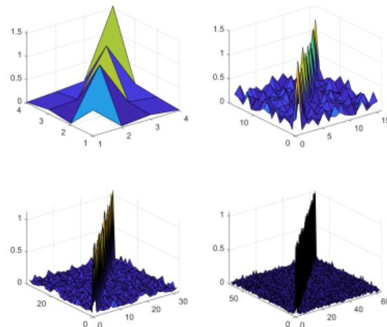
Figure: The magnitudes of  $\mathbf{H}^H \mathbf{H}$  for different RIS elements, namely,  $N = 4$ ,  $N = 16$ ,  $N = 32$ , and  $N = 64$ .
