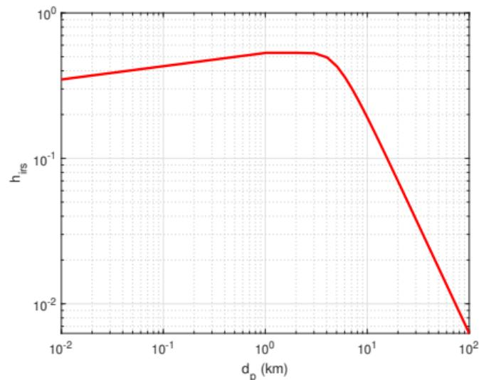
Figure: GML for IRS-based FSO channel between LS and PD versus  $d_p$
