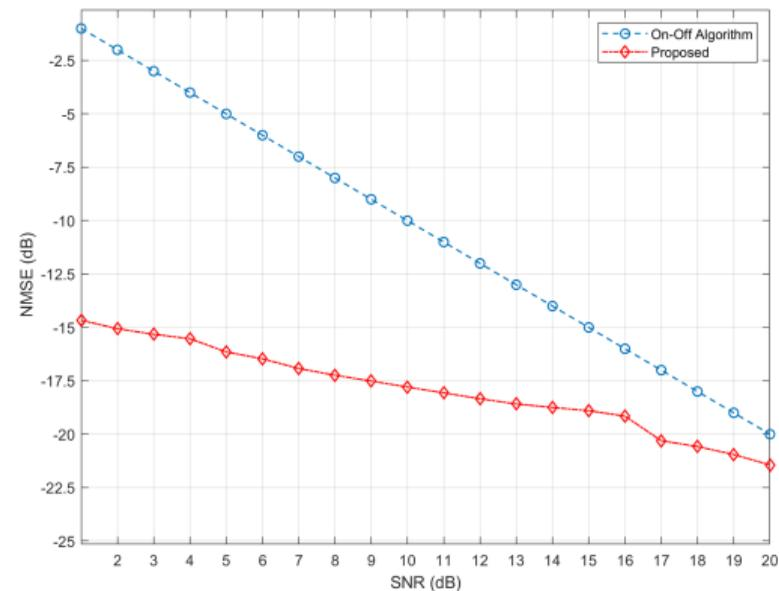
Figure: The NMSE vs SNR with  $\zeta = 0.2$  and  $\frac{d}{\lambda} = 0.1$ .
