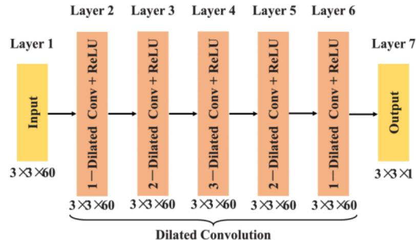
Figure: Stage Two: the proposed STS-CNN model
