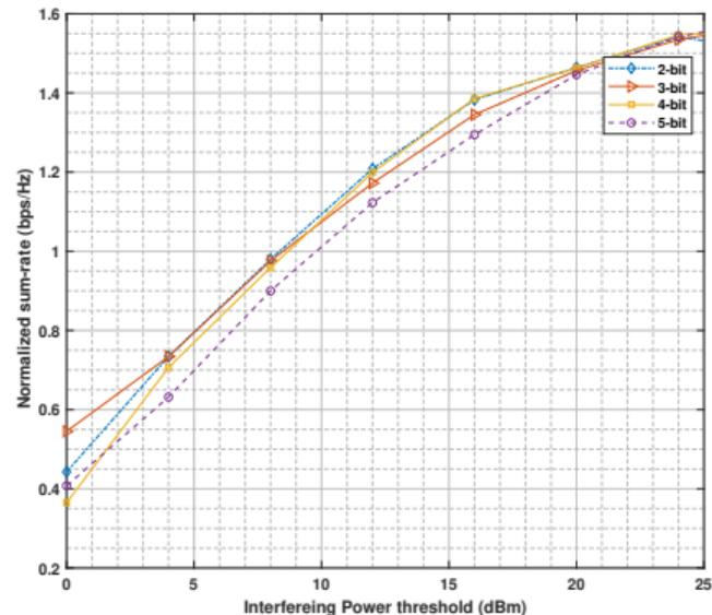
**Figure:** The achievable sum-rate  $R$  vs the radar interfering power threshold.
