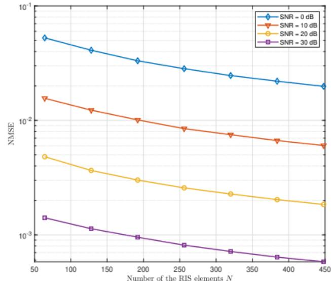
Figure: The NMSE of F vs. number of RIS elements for different SNR values when  $M = 32$ .
