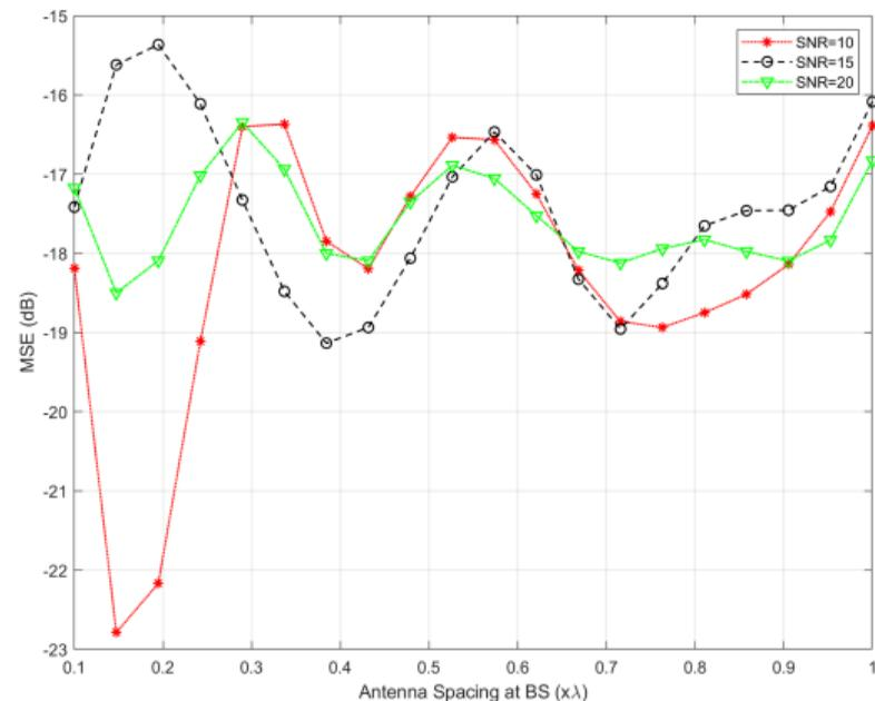
**Figure:** The effect of Antenna spacing at the BS on the NMSE performance of the proposed approach.
